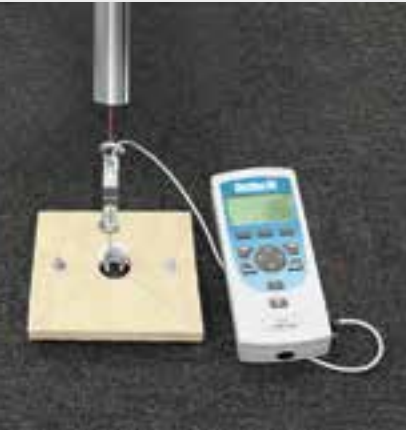
Testing of fixing element strength
